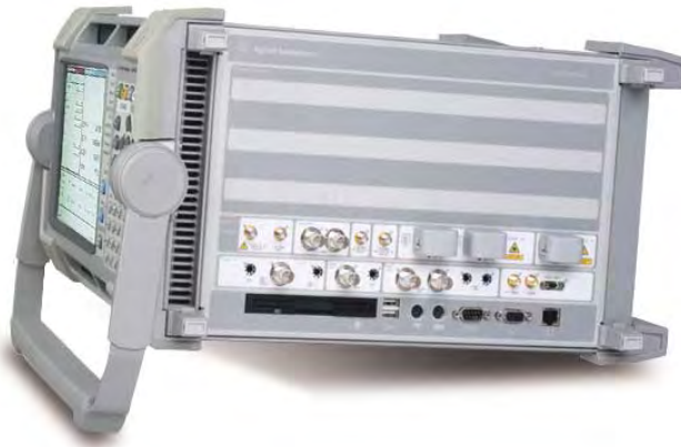
OmniBER OTN 2.5 Gb/s communications performance analyzer with Ethernet over SONET/SDH support
